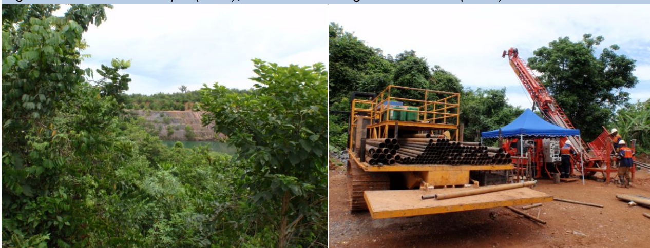
Fig. 9: Adubiaso mined pit (LHS); Diamond drilling at Adubiaso (RHS)
